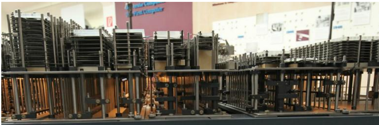
Fig. 2: The mechanical layers of the Z1. The eight memory layers can be seen on the right, the 12 processor layers on the left. The lower section with levers is used for transmitting the clock cycles to all parts of the machine.
